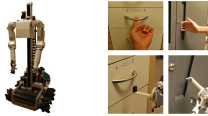
Fig. 2. Left: The mobile manipulator used in this work. Right: Examples of a human using his hand as a hook and corresponding orientations for the robot’s hook end effector.
